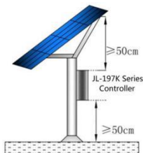
Figure 4. Control Box Location
