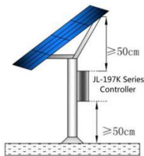
Figure 4. Control Box Location
